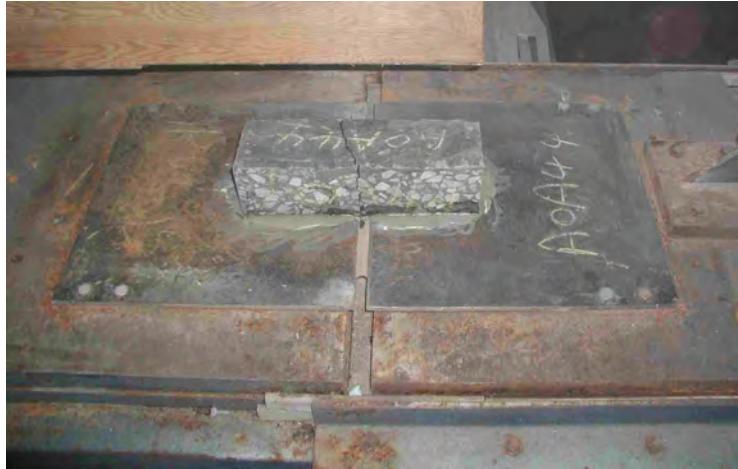
Figure 7: Specimen in Static/Cyclic Direct Tensile Strength Test.
